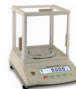
**Fig 6: Shielded Electronic Chemical Balance**
